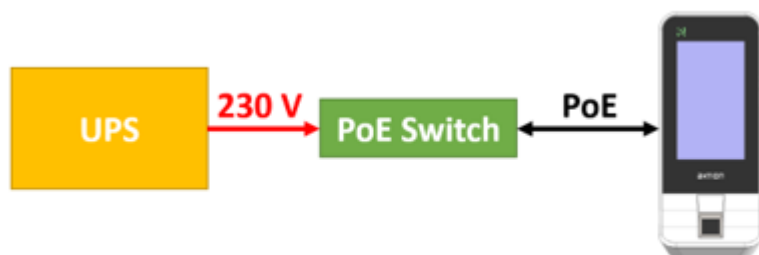
Obr. 6: PoE switch s UPS
