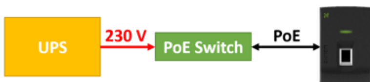
Obr. 5: PoE switch s UPS
